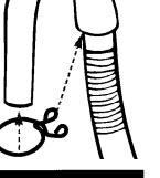
Before attaching water inlet hose, run water through both faucets into a bucket. This will get rid of particles in the water lines that might clog hoses. Mark which is the hot water faucet.
